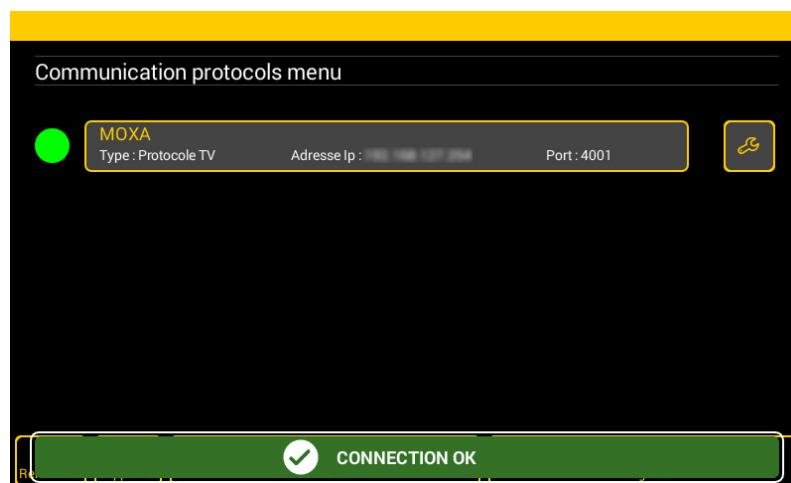
8) Start the chosen sport and the match. The protocol will be emitted automatically on the serial port of the interface.
