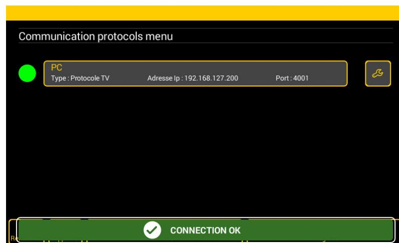
8) Start the chosen sport and the match. The protocol will be automatically transmitted on the RJ45 output.
