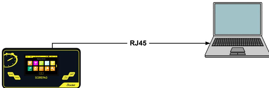
**2 : from the RJ45 port of the Scorepad to the RS232 com port of the external PC via an RJ45/RS232 interface.**
