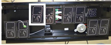
3/ Attach the DIN connection cable between the scoreboard and scoreapp (ref.: 408901):
