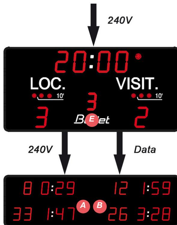
Most of the cabling for the BTX6125HK is carried out at the factory. This guide only covers the cabling required on installation. All cables to be attached are located around the sides of the BT6102E: 1 power supply with a green connector (240V) and 1 communications cable with a green connector (DATA).
