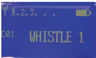
Channel number, whistle number, battery charge and number of terminals in the network
